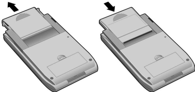
The Backup Module includes complete backup and restore software that lets you make secure copies of your valuable handheld data with the touch of one button. Restoring your data is just as easy.
