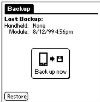
Tapping the Back Up Now button initiates a backup of all data on the handheld. The software displays a progress bar as it copies data to the module.
