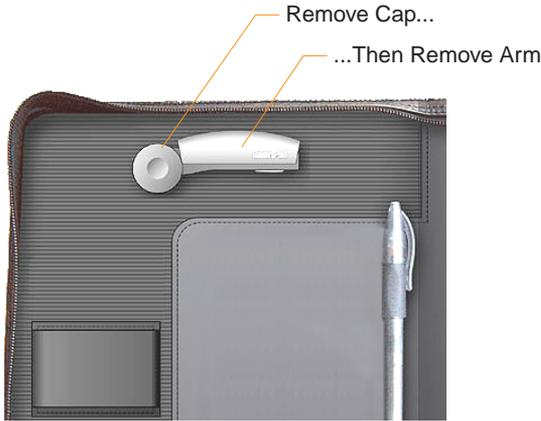
3. With the round cap removed, carefully pull straight up to remove the arm of the infrared transceiver from the snap retainers of the SmartPad portfolio. Be aware that a wire connects this arm to the SmartPad portfolio — take care not to pull on the wire as you remove the arm of the infrared transceiver..
